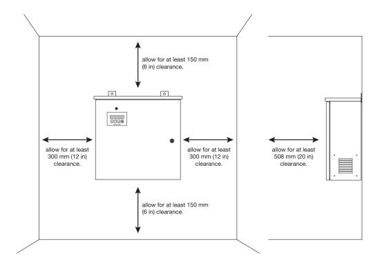
Figure 2.3 Minimum Clearance for Proper Mounting
